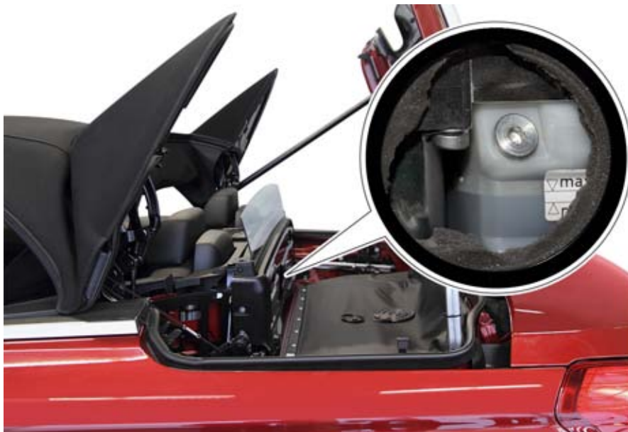
F12 Hydraulic fluid reservoir, service openings
