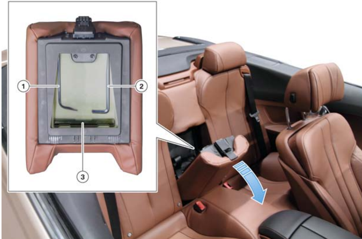
F12 Tools for emergency operation of soft top
