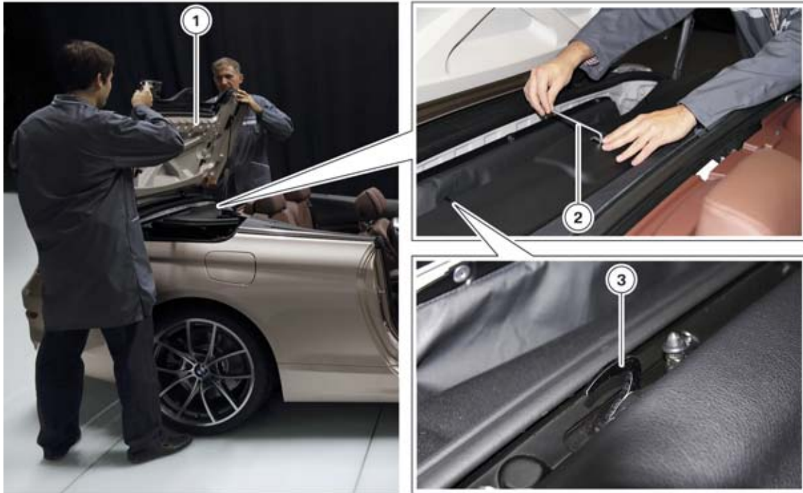
F12 Opening the soft top compartment lid and releasing the cowl panel lock
