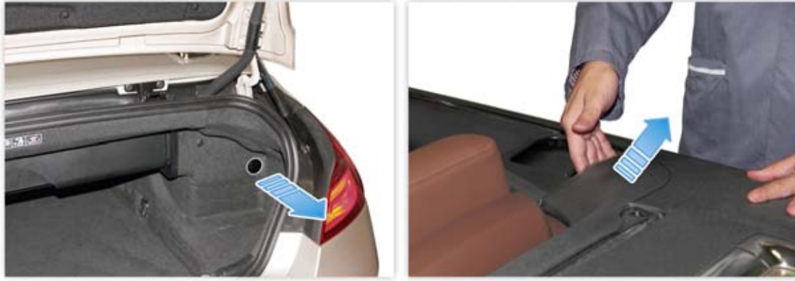
F12 Unlocking the soft top compartment lid
