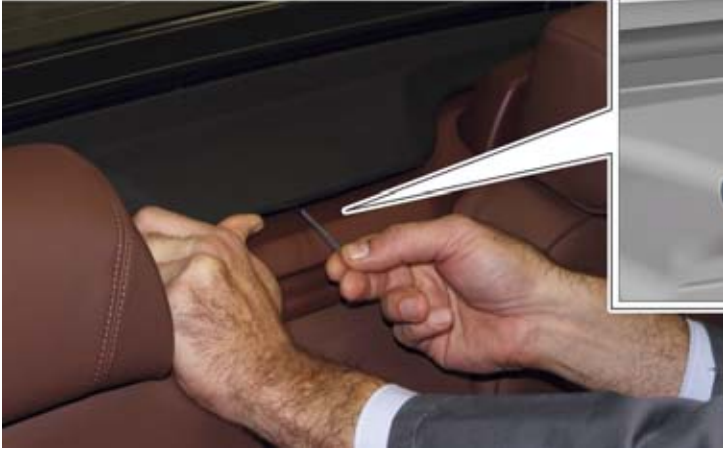
F12 Manually lowering the rear window
