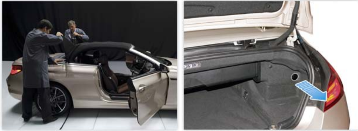
F12 Unlocking the soft top compartment lid
