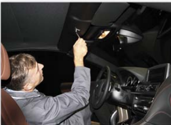
F12 Unlocking the soft top on the cowl panel
