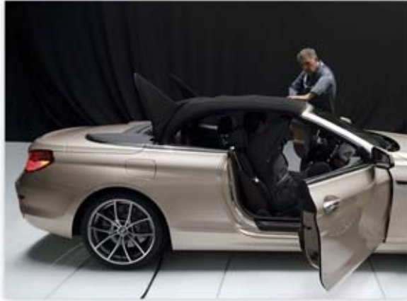
F12 Locking the soft top on the cowl panel
