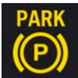
F12 Indicator light showing parking brake fault
