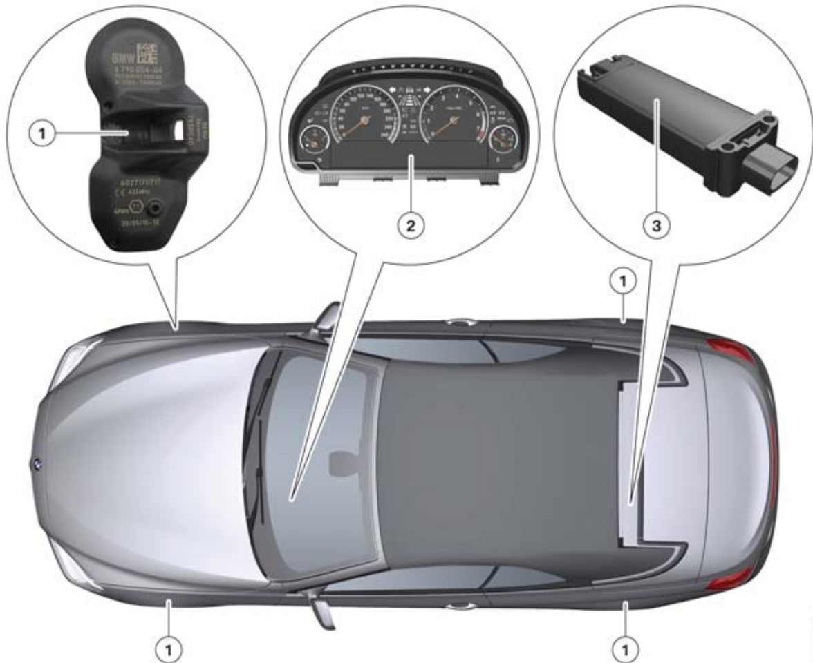
F12 System overview of TPMS
