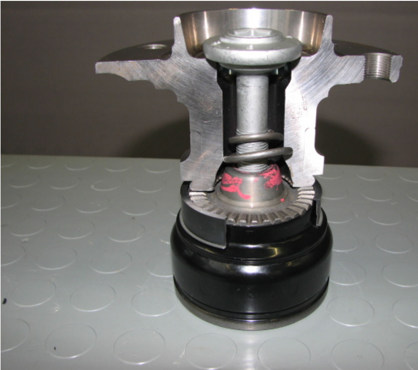
Cutaway view of the new front axle spur gear connection to the wheel hubs
