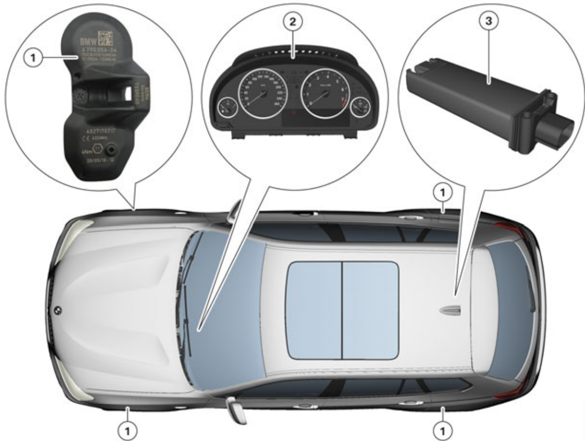
F25 System overview of TPMS
