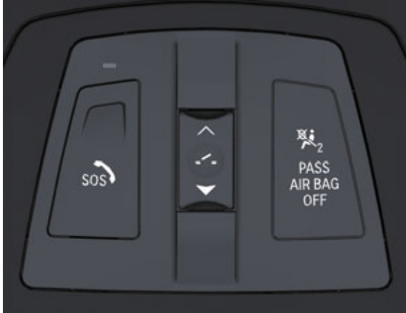
F25 Roof function center with indicator lamp for front passenger airbag deactivation
