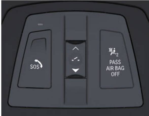
F25 Roof function center with emergency call button
