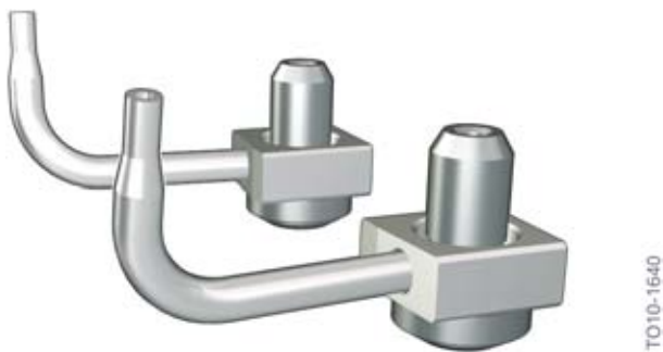
N20 engine, oil spray nozzles for piston crown cooling
