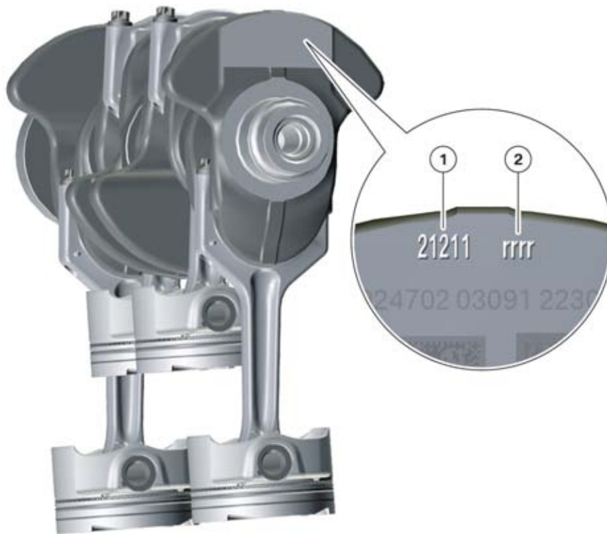
N20 engine, bearing identification, crankshaft code
