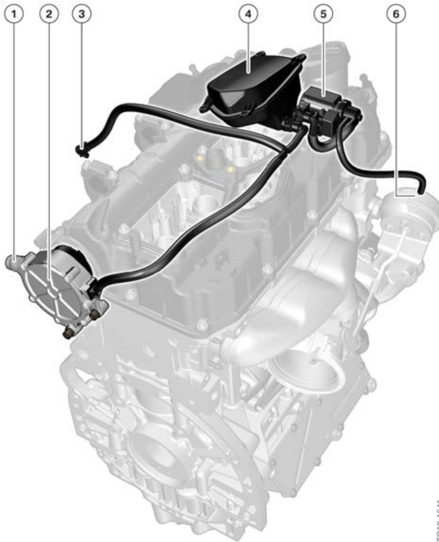
N20 engine, vacuum system
