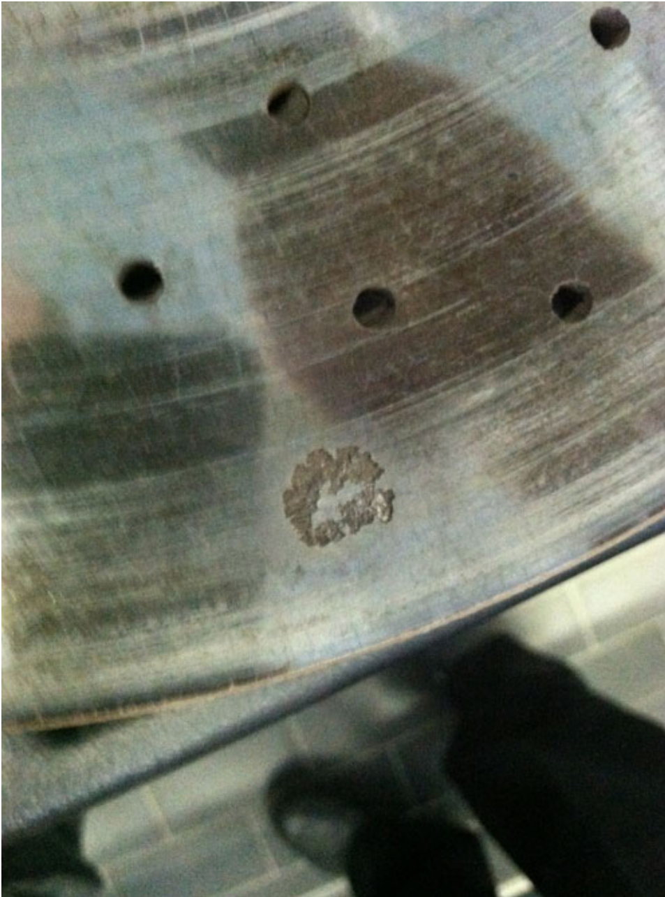
Disc must be replaced, total wear
