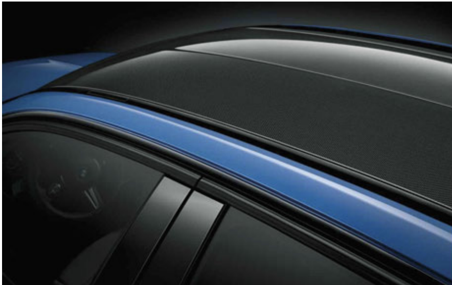
F80 M3 CFRP roof
