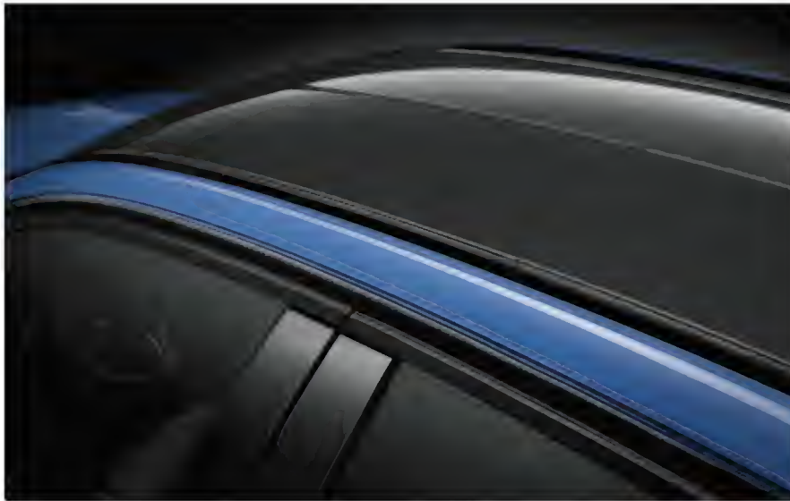
F80 M3 CFRP roof
