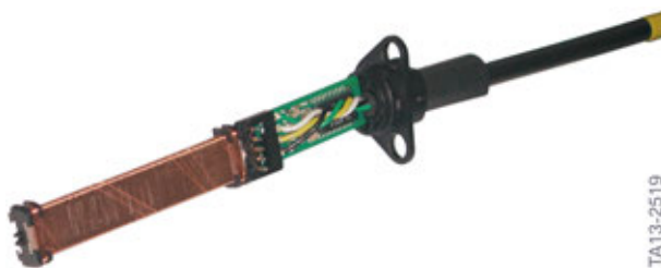
Example of a PLCD sensor (from clutch slave cylinder E60 M5)
