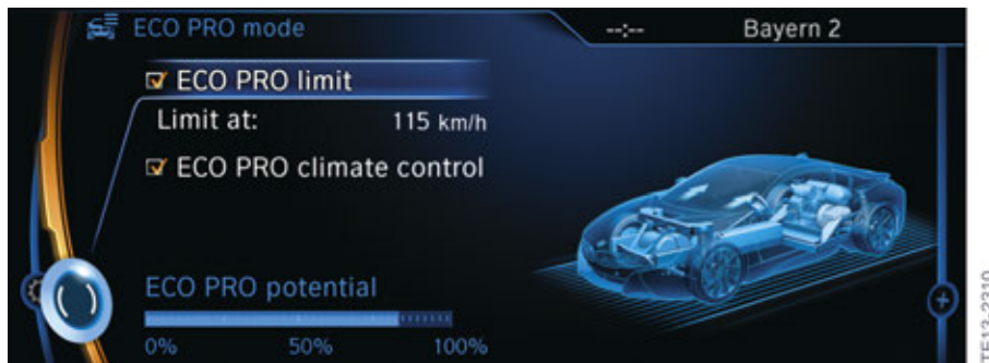
I12 Power reduction of heating/air-conditioning system
