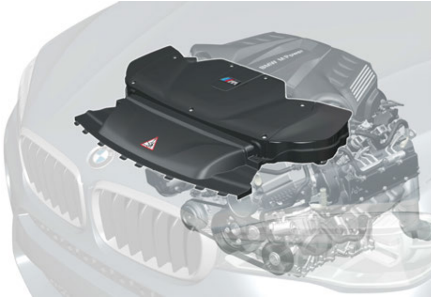
F85/F86 M air intake duct and intake silencer
