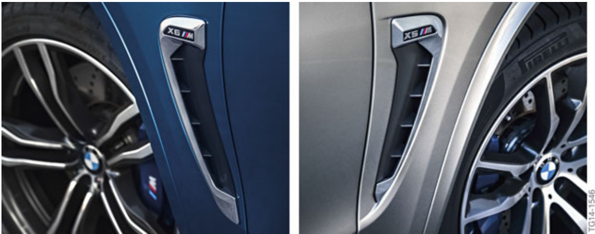
F85/F86 M gill elements with integrated air breather
