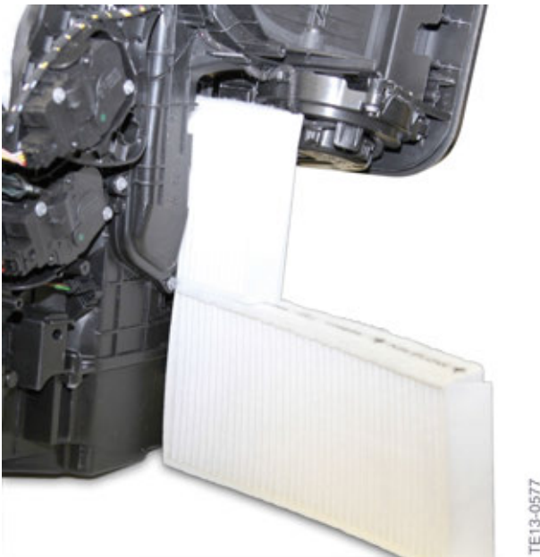
F48 heating and air-conditioning unit, replacement of microfilter
