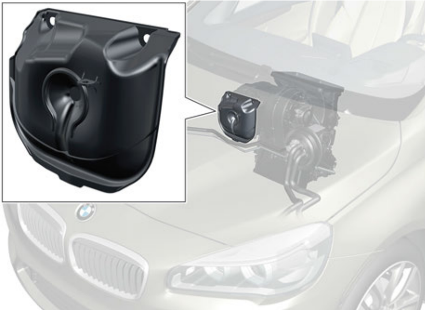
F48 air/water separation (Venturi adapter)
