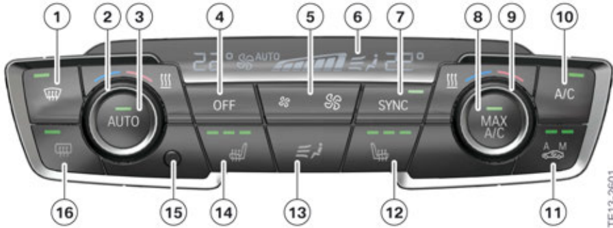
F48 IHKA control panel
