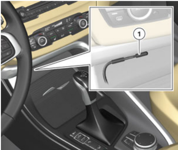
F48 installation location of Bluetooth antenna
