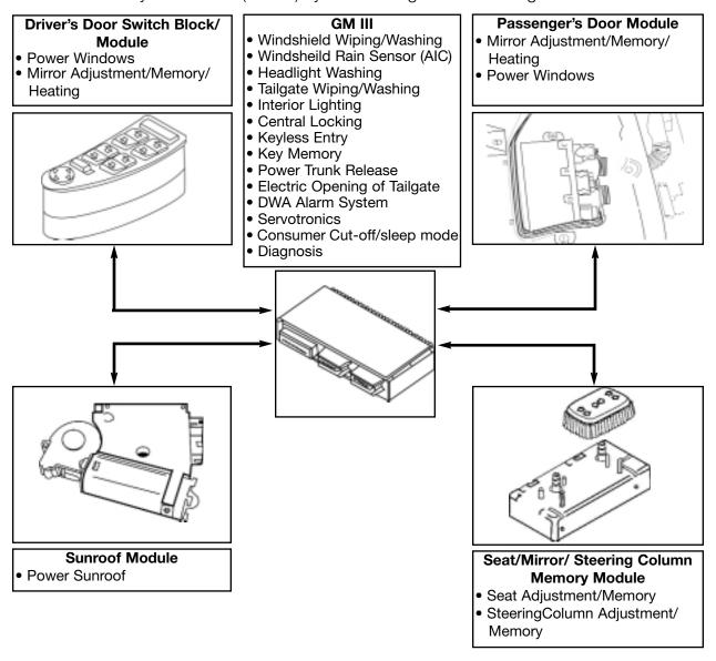
The ZKE III system was introduced on the E38 and is used in the E39 and E53. Most of the functions operate the same on these vehicles with minor changes and added features to the system.
