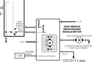
Pressing the wiper stalk forward to the first detent activates the rear wiper in the intermittent mode. The timed interval is approximately 7-12 seconds. The full sweep and park positions are recognized by the two hall sensors on the motor gear assembly. If the wiper is switched OFF, the wiper blade will return to the park position.
