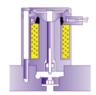
**Electro-Hydraulic Solenoid Control:** The GM monitors the road speed input and supplies the electro-hydraulic solenoid with power. The road speed signal "A" is supplied from the IKE (and K-Bus) on E38 vehicles and from the DSC Control Module on E39/E53 vehicles.
