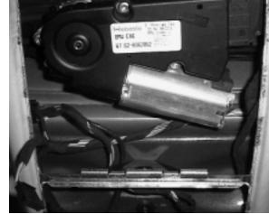
The electronic controls and relays are contained in the sunroof module (PM-SHD). The module is connected to the P-Bus (E38 >99 MY on the K-Bus) for comfort closing/opening and diagnosis/fault memory purposes.
