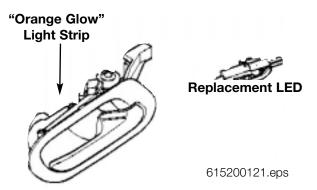
The LED's are connected to the KL 58g interior panel lighting circuit. KL 58g is an output pulse width modulated control signal from the LCM III. The duty cycle changes when the LCM III detects a change in the voltage drop at the light dimmer input signal.
