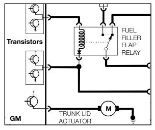
The ZKE III system offers an overall reduction in vehicle wiring particularly in the areas subject to wear from movement such as doors, seats and the steering column. To accomplish this, the "P- Bus" is used to interface (signaling) with peripheral modules over a single wire. The ZKE III modular system consisting of the following components:
