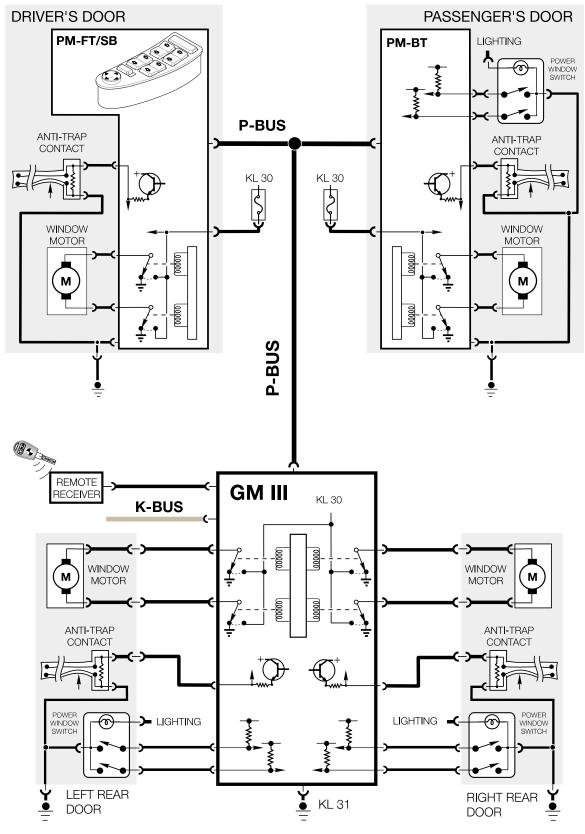
**Power Window Motors:** The window motors are mounted on the cable regulators. The window motor control circuit consists of two wires for operating the motor in both directions.
