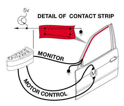
The example shown represents the driver's door window control and monitoring carried out by the Driver's Door Switchblock Module (PM- FT/ SB).
