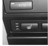
• All three LEDs illuminate and the heating elements are provided regulated output current producing a seat temperature of 111°F.
