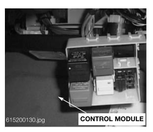
The GM controls the soft on/off feature of the vehicle interior lights by a pulse width modulated control signal. This signal is also an input to the Visual Entry Aid control module which requests simultaneously control (soft on/off) each exterior door light source.
