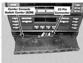
The switch signal output for these systems is a direct output signal. All diagnosis functions are carried out through their respective control systems.
