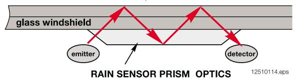
The density of water is closer to that of glass than air. When rain starts to accumulate in the sensor monitoring area, it causes part of the infra red beam to extend past the outside surface of the glass and into the rain drop. When this occurs, the beam is refracted and only part of the beam returns to the detector diode.
