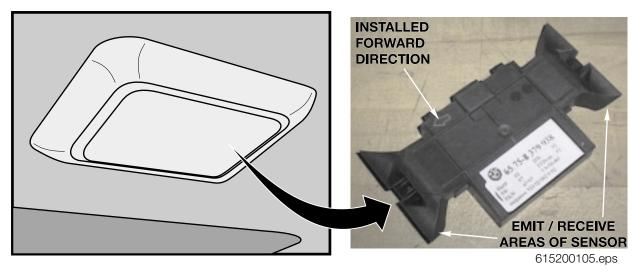
Every time the DWA system is armed (signal STDWA), the sensor adapts to what ever objects might be stationary in the interior. The sensor emits ultra sonic waves in a programmed timed cycle. It receives echos of the emitted waves.
