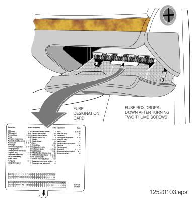
The placement of the power distribution box is close to the main electronics carrier **behind the glove box**. The modules/relays located in the electronics carrier include (examples):
