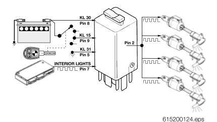
**Light Source Modules:** Mounted in each door are the light source modules.
