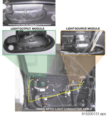
**Light Output Modules:** The exterior door handle frames have an additional mount to accept the light output module.
