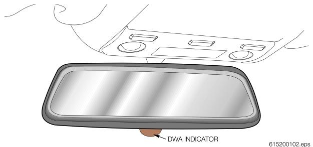
The system is "armed/disarmed" from the driver's door lock cylinder, remote transmitter or luggage compartment lock cylinder. The alarm is immediately deactivated when disarmed with the key in the driver's door lock cylinder (may be deactivated in Conversion) or remote transmitter.
