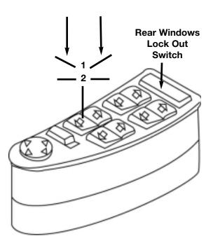
All window operations signals are digital inputs to the door module and GM III.
