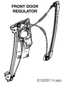
**Window Motor Limit Stop Function:** If the windows are run up and down continuously a limit stop function is activated to prevent the window motors from overheating. The GM monitors the number of times the window motors are activated. Each cycle is counted and stored in memory.
