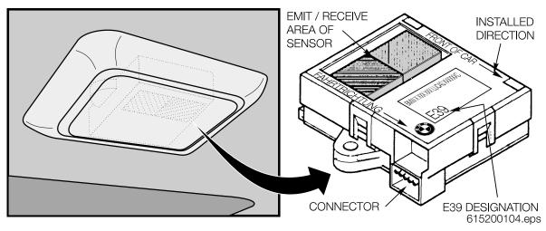
When the alarm system is armed, the sensor emits electromagnetic waves at a frequency of 2.45 GHz. As long as nothing is moving in the vehicle, the waves as bounced back to the sensor at the same frequency. The sensor monitors these bounced back waves as an indication that nothing is disturbed within the vehicle.
