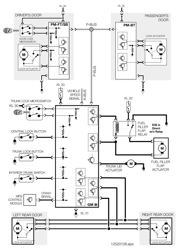
**Door Lock Actuators:** A door lock actuator contains an electric motor and an integrated microswitch (position switch). The rotary motor movement through the gear drive mechanically moves the locking latch.
