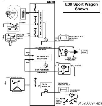
Rear window unlatching is requested by the rear window switch ground signal. This signal initiates activation of the rear window actuator relay control circuit which activates the rear window actuator. The actuator unlatches the mechanism opening the window. The latch simultaneously provides an open window signal for the rear window wiper motor module as well as an interior light on request (via the wiper module).
