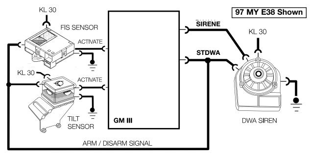
The activate siren signal to the siren is high whether DWA is armed or disarmed. If a monitored input activates the alarm, the high signal to the siren is switched to a 50% duty cycle at the GM. The control circuitry in the siren activates the siren driver.
