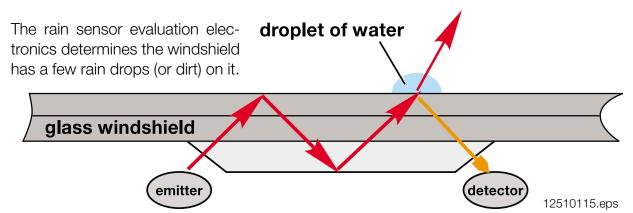
The intensity of the returned infra red beam diminishes proportionally with an increase of water droplets. The rain sensor control module generates a signal proportionate to the amount of rain on the windshield and broadcasts it to the GM via the K bus.
