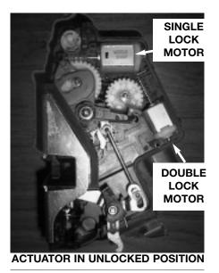
WHEN IN DOUBLE LOCK AN INTERIOR ACTUATED UNLOCK ROD IS OFFSET PREVENTING THE LOCK MECHANISM FROM BEING MECHANICALLY UNLOCKED
