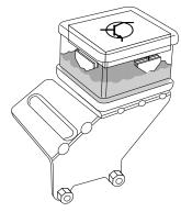
DWA ARMED, TILT SENSOR REGISTERS RESISTANCE VALUE THROUGH FLUID. SIGNAL HIGH TO GENERAL MODULE
