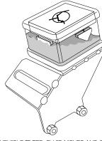
VEHICLE TILTED, FLUID MOVES AND CHANGES RESISTANCE VALUE BETWEEN PLATES. HIGH SIGNAL MOMENTARILY GOES LOW SIGNALLING GM TO ACTIVATE THE ALARM.
