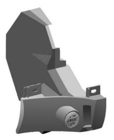
The CAS is the Gateway between the K-CAN System and K-CAN Periphery Bus.
