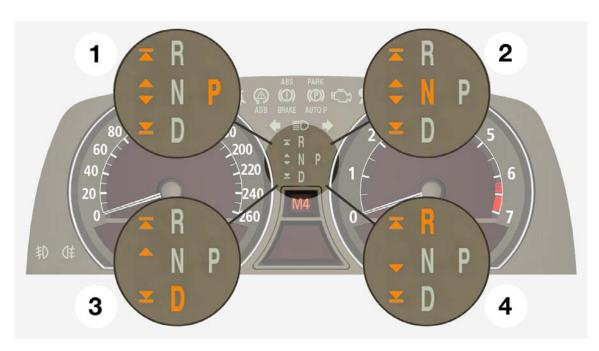
The arrows beside the program display indicate each of the possible directions of movement of the transmission selector lever. The program display remains illuminated for 10 seconds after the remote control has been removed (after-run function).
