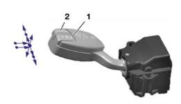
Briefly tapping the lower button (1) scrolls all the display options in the display area below the speedometer.
