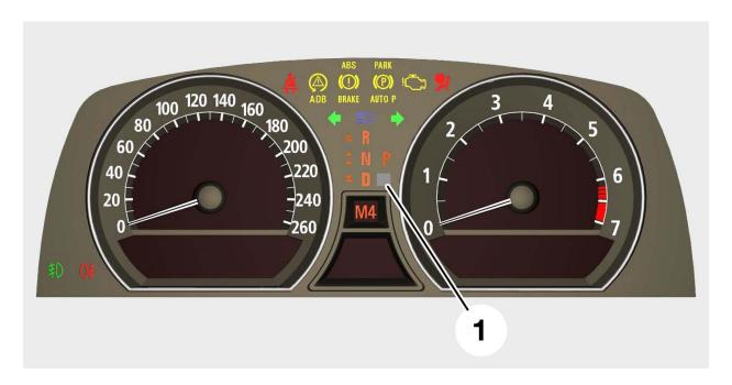
The brightness signal is calculated in the instrument cluster from the values of the photo-transistor (1) and the dimmer wheel. This brightness signal is also made available via the K-CAN System to other control units in the vehicle. The instrument cluster is thus used as the "dimming master".
