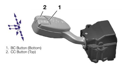
The CC button in the turn signal stalk can be used to browse through all the CC messages issued (press briefly), or to toggle between the On-Board Computer and Check Control in the display area below the tachometer.
