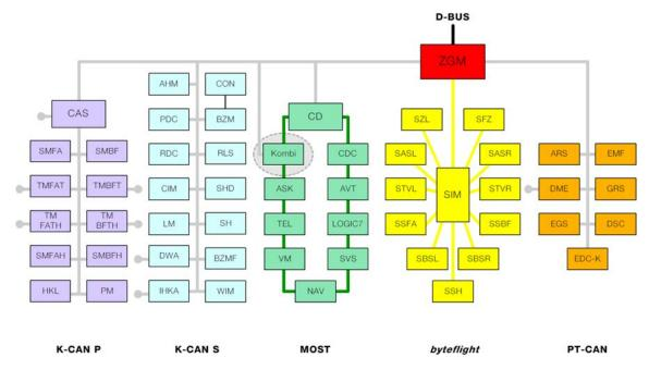
The communication with control units in the chassis, power train and body areas is via the K-CAN System.
