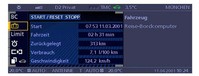
The travel computer displays the starting time and date, driving time, distance travelled, average fuel consumption and average speed exclusively in the Control Display.
