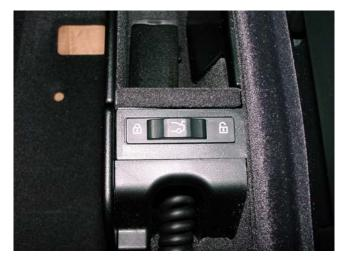
When the setting is "locked", the interior and outside trunk release button inputs are ignored.
