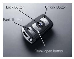
Up to four Remote Controls may be assigned to the vehicle for remote services (not EWS which may have up to 10). There is no procedure necessary for initialization, once the EWS transponder of the Remote Control is identified by the CAS, the radio frequency transponder is also logged in as valid.
