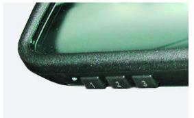
grammed channel button. The integrated universal remote control uses radio frequencies only (not infrared). Transmission of the signal is indicated by the indicator LED.
