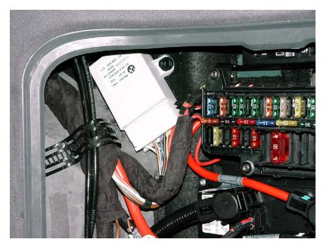
The Power Module controls the operation of the trunk lid lock and the soft close assembly as well as signalling (over the K-CAN P) the requests for opening and closing the trunk from the external trunk button.
