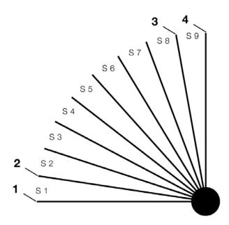
Shortly before reaching the end stop "lid open" (transition from segment 7 to segment 8), trunk speed is reduced and the lid slowly moves to its end position.
