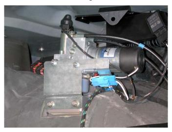
It is controlled via a PWM signal from the HKL control unit. The signal is varied depending on the opening angle of the trunk lid to maintain an even closing speed over the entire range.
