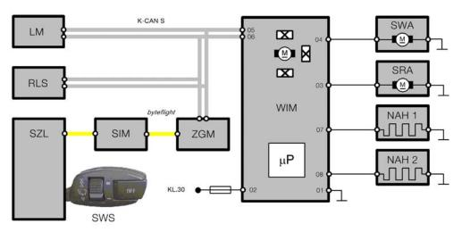
Note: If communication between the wiper switch and the wiper module is disturbed, the failsafe result is continuous operation of the wipers.
