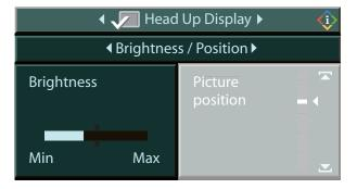
The brightness setting is automatically corrected in order to compensate for different light conditions. Compensation is based on signals from the rain and light sensor. The automatic brightness setting is configured in such a way that no HUD brightness jumps occur.
