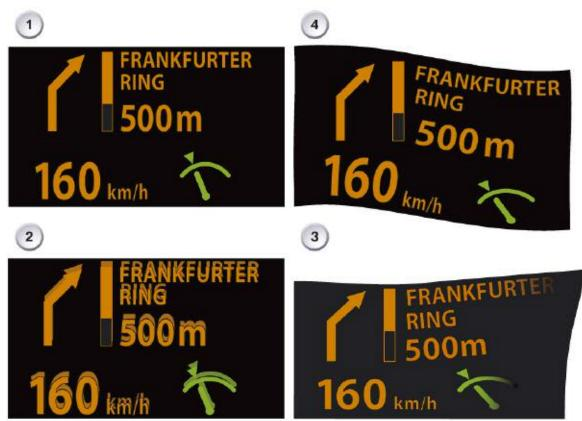
Image 1 is compressed widthways. Image 2 is displayed twice. Images 3 and 4 are distorted.
