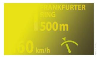
Note: It is only possible to adjust the head-up display vertically (rotation) and correct the image in the event of distortion (warping) using the BMW diagnostic system. Detailed information on the subject of Warping may be found in the BMW diagnostic system.
