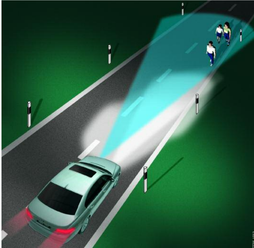
Comparison of BMW Night Vision Visibility with Different Vehicle Headlights
