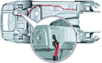
Within the battery box are two transfer points (as shown) for the two cables that run to the engine compartment.
