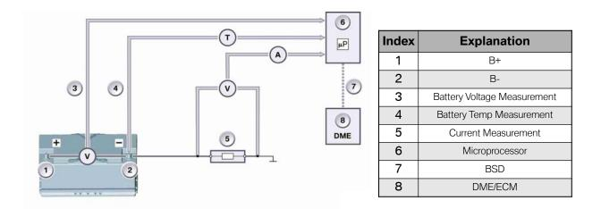
The IBS is able to withstand thermal loads up to 105°C, the chemical effects of the battery acid.
