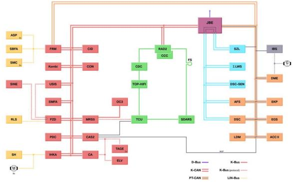
Control Modules Connected To Terminal 30
