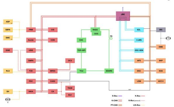
Control modules connected to Terminal 30g\_f
