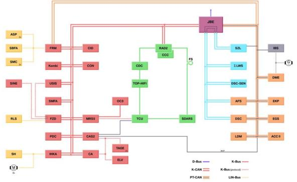
Control modules connected to Terminal 30g
