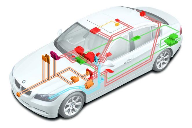
Main bus systems are responsible for the data exchange between the control modules throughout the vehicle system.
