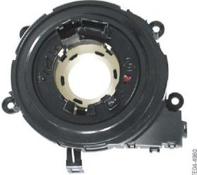
The front wheels and steering wheel must be set to the straight-ahead position as the prerequisite for disassembly. During disassembly of the steering wheel, the load on the lock pin of the coil spring assembly is relieved and the pin can lock in the straight ahead position.
