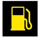
The fuel reserve level is not indicated by an indicator lamp as in the previous models. A fuel pump symbol lights up for 23 seconds in the liquid crystal display as soon as the reserve level is reached (2.1 gallons).
