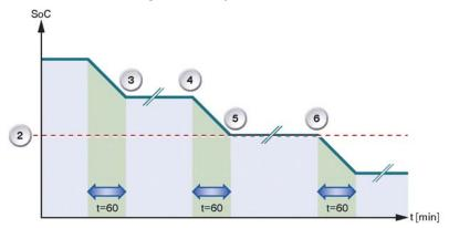
As of 3/2005 - The improvement of the new deactivation strategy becomes apparent with a renewed activation of the loads/consumers (by a terminal change or unlocking of the car) in the event of a previously ascertained closed circuit current violation or an extended starting capability limit which has already been reached.
