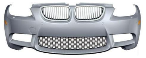
Front bi-xenon headlamp units are identical to the series E92. The M3 front bumper overhang is longer than that of the series E92.
