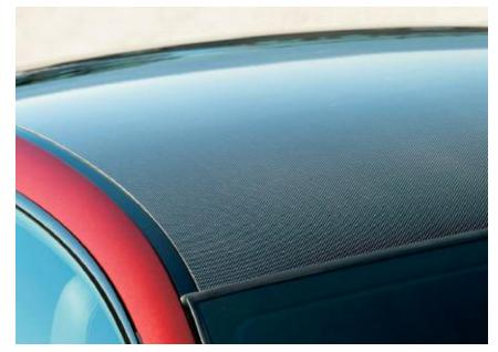
The carbon fiber-reinforced plastic roof is 7 kg lighter than the standard steel roof therefore lowers the vehicle's center of gravity. This has a particularly positive effect on the vehicle dynamics.
