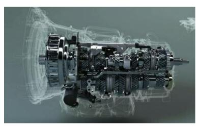
M-DCT Dual Clutch Transmission
