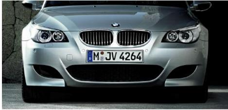
In conjunction with sealing the engine compartment, the front bumper reduces lift on the M5's front axle by 50% in comparison to the standard car.
