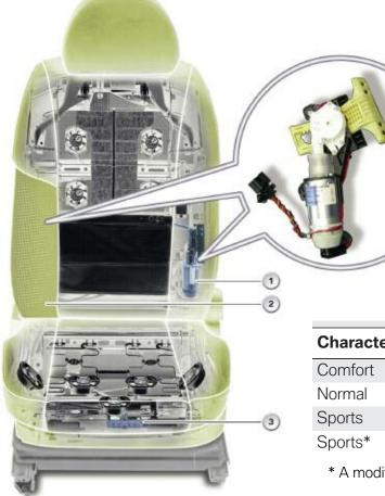
The active backrest width adjustment system consists of the following control units:
