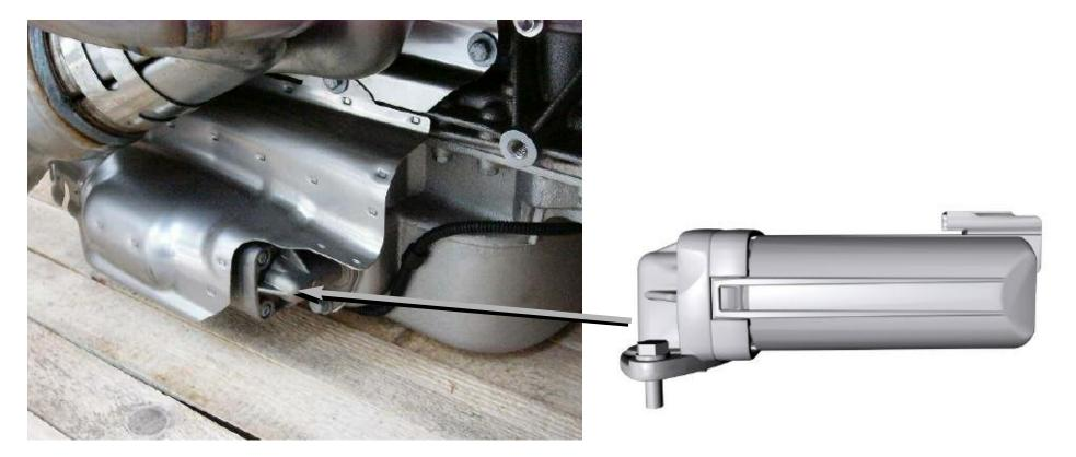
Electrically operated "duo-centric" oil pump (Left side shown)
