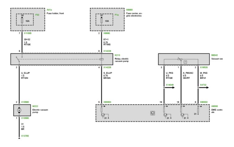
A test module is provided in ISTA/GT1 for the electric vacuum pump. The differential pressure sensor on the brake booster is used for the purpose of monitoring the pump.
