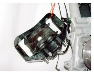
**Dual Piston Front Brake Caliper**
