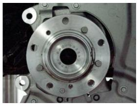
**Detail of Rotor Alignment Pins on Hub**
