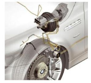
Mounting Location of DSC Control Unit and Hydraulic Unit
