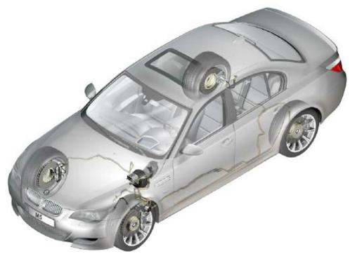
measures the pressure from the tandem master brake cylinder THZ and four further sensors that measure the braking pressure of the respective wheel brake.
