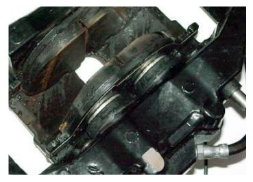
**Dual Piston Front Brake Caliper (close-up view)**
