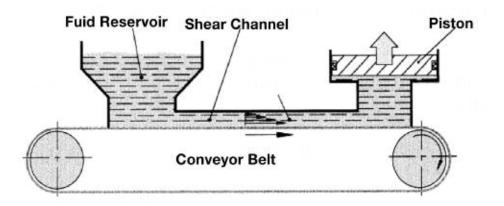
By transferring the operation principle to a rotary system, the conveyor belt becomes a displacement disc driven by the Hub. The shear channel is then a circular groove in the control disk. The control disk is located in the pump housing.
