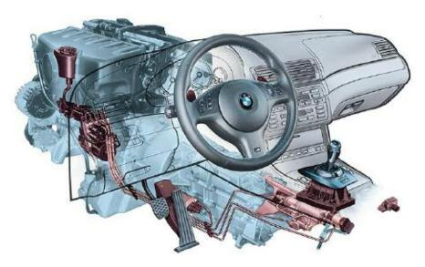
E46 M3 SMG 2 Shift/Clutch Mechanism
