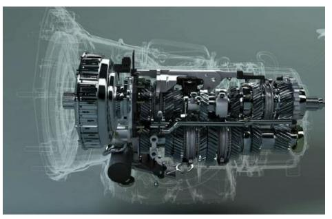
E9X M3 M DCT transmission cut away view
