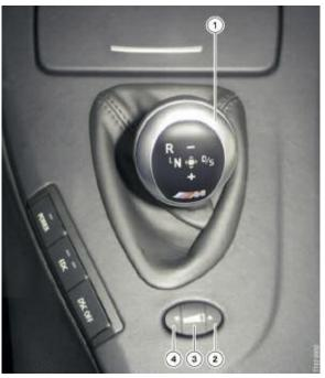
M DCT M Gear Selector Switch (M GWS)
