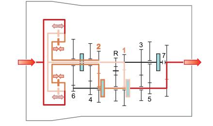
M DCT gear shift from 1st to 2nd gear, third phase
