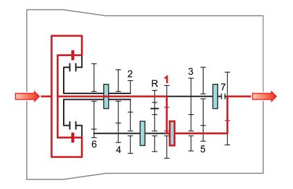
M DCT power flow route 1st gear
