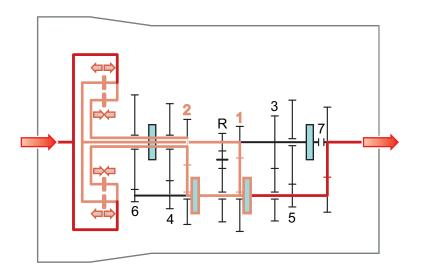
M DCT gear shift from 1st to 2nd gear, second phase
