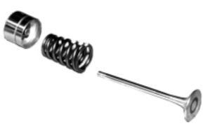
The springs are marked for correct installation due to the "cone" shape (paint stripes facing down towards cylinder head).
