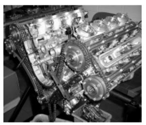
**Camshaft Secondary Drive:** Secondary drive is from the intake camshaft to the exhaust camshaft by a single roller chain (arrow). The chain is tensioned by a hydro-mechanical "self adjusting" tensioner (between the sprockets).
