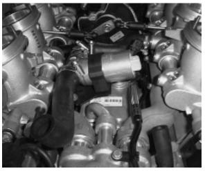
**Fuel Supply:** The fuel is supplied through a Non Return Fuel Rail System. This system is used on the S62 for TLEV compliancy. The fuel supply pressure is controlled by the 5 Bar fuel pressure regulator integrated in the fuel filter assembly (pressure test fitting at this point). The E39 M5 fuel filter assembly is located under the left front floor area (next to the frame rail).
