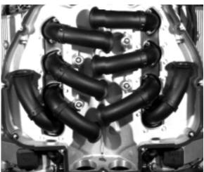
**Intake Air System:** The S62 engine uses eight individual throttle housings that are bolted directly to the cylinder heads. To ensure smooth and stable engine operation all eight throttles must be synchronized for an even distribution of the intake air.
