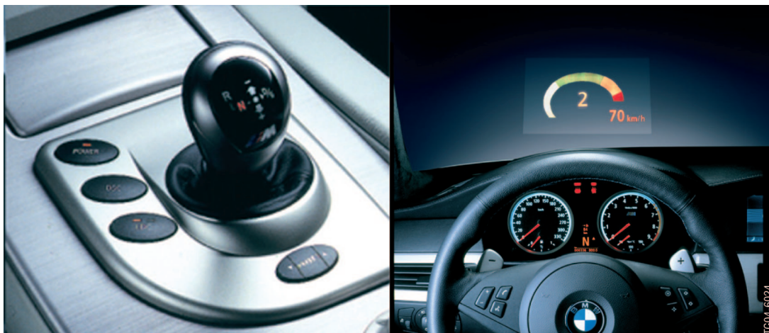
1 - Selector lever and head-up display in the E60 M5
