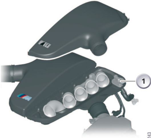
25 - Cyclone separator (1) in intake air manifold
