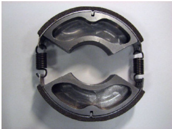
Clutch Material with Springs and Weights
