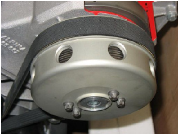
Bell Housing/Pulley Installed
