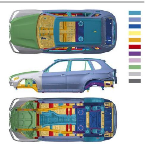
The various colors in the above illustrations show the variety and mix of materials used on the E70. These materials are advanced steels which are used according to the requirements such as strength, weight and thickness.
