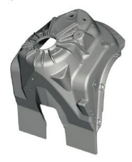
The cast aluminum spring support (strut tower) of the E70 is distinguished primarily by the following features:
