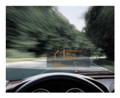
The separate components of the head-up display are the cover glass, 2 mirrors, LED power supply, LED array, TFT projection display, PCB and casing. The head-up display can only be replaced as a complete unit. It is not possible to replace components or separate parts.
