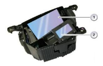
The convex mirror (1) is responsible for compensating the image on the windshield and for the size and distance of the image.
