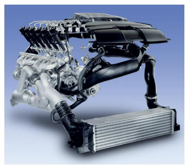
The turbocharger consists of a turbine and compressor assembly (1) on a common shaft inside of the turbocharger housing. The turbine wheel is driven by waste exhaust gases and in turn drives the compressor wheel.
