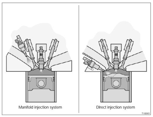
The DI system allows for increased engine efficiency and has several distinct advantages over manifold injection systems:
