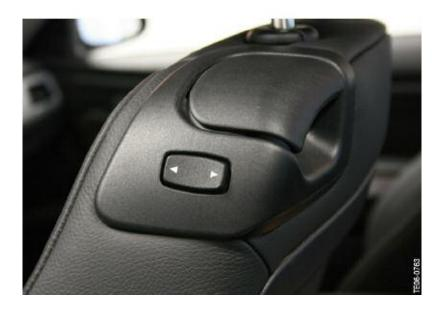
When entering the rear compartment, the customer can move the seat forward with the adjustment switch. By mechanically releasing the seat backrest, it can be additionally tilted forward to create sufficient space for convenient entry.
