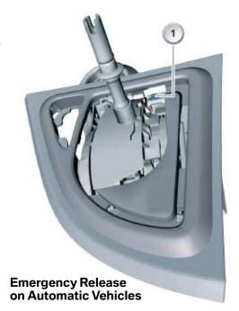
The ELV cannot be dropped on automatic transmission vehicles as these vehicles do not feature an emergency release facility for the selector lever with the key.
