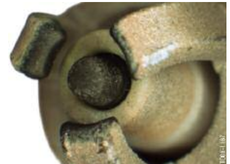
Spark plug showing normal wear pattern for high mileage
