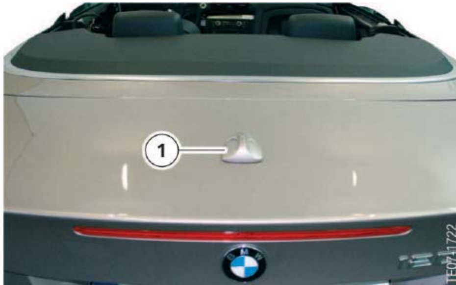
Satellite Digital Audio Radio Services (SDARS) antenna on trunk lid (View from the rear of the vehicle)
