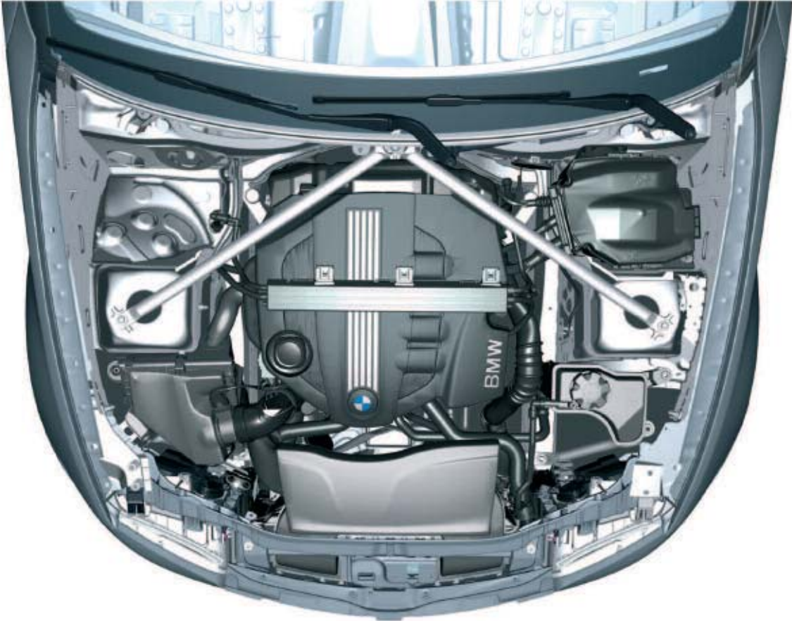
Top view of front shock tower bracing (hood removed)
