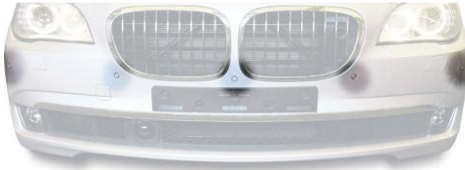
F01 front bumper with five Park Distance Control ultrasonic sensors
