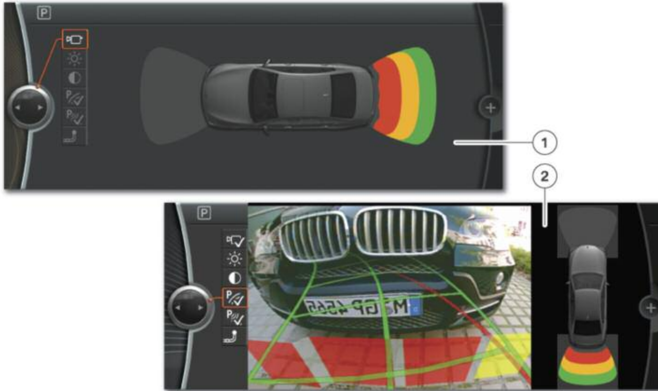
Distance warning PDC display and option to select rear view camera image with PDC
