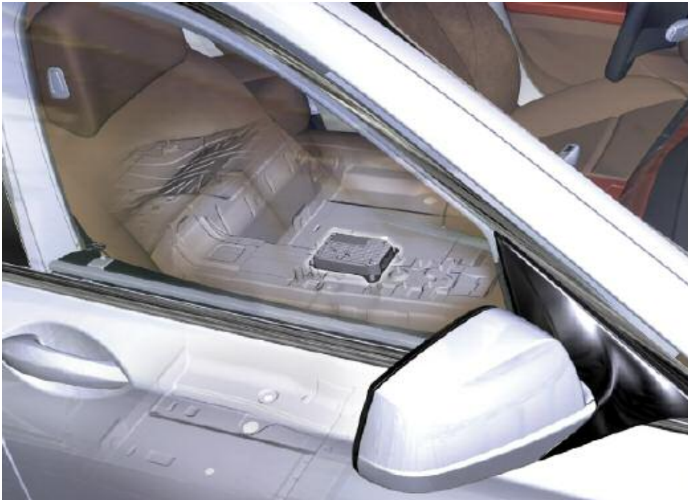
Installation location of the ICM control unit overview
