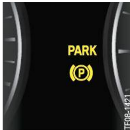
Indication of “parking brake emergency release/fault”
