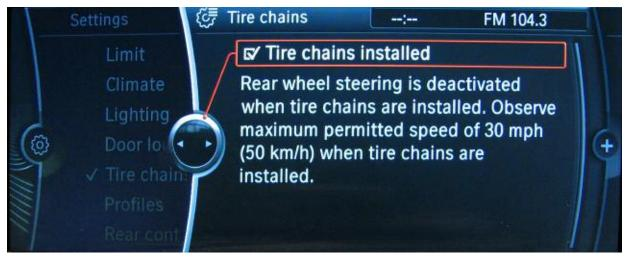
When show chains are used, the setting on the iDrive Settings menu must be changed to "Show chains fitted".
