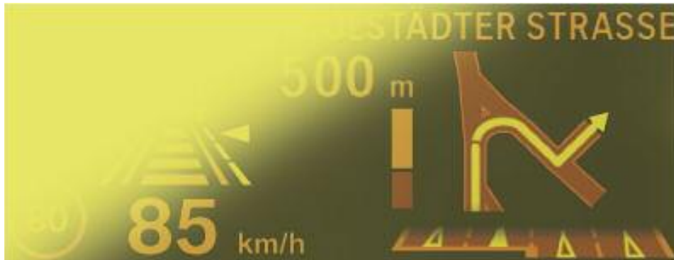
Image defect caused by incident light or overheating in the HUD
