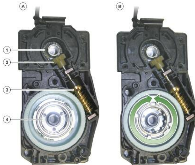
Drive unit with separate components (A) and freely rotatable ring gear (B)
