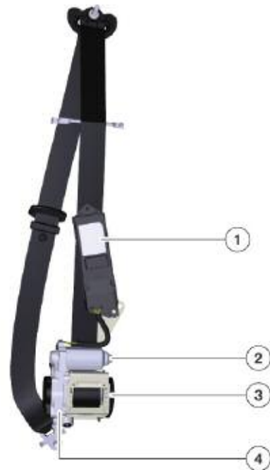
Seat belt with electric motor driven reel
