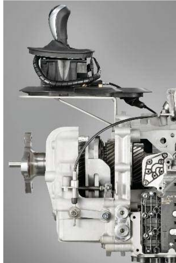
M DCT parking lock lever, (cut away view from rear right of transmission)
