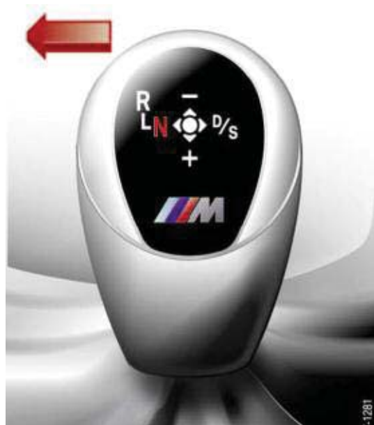
The M GWS one-touch function is pushed to the left to shift into neutral.
