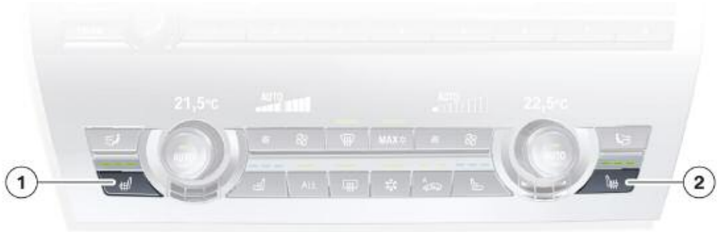
F07 integrated automatic heating and air conditioning system control panel
