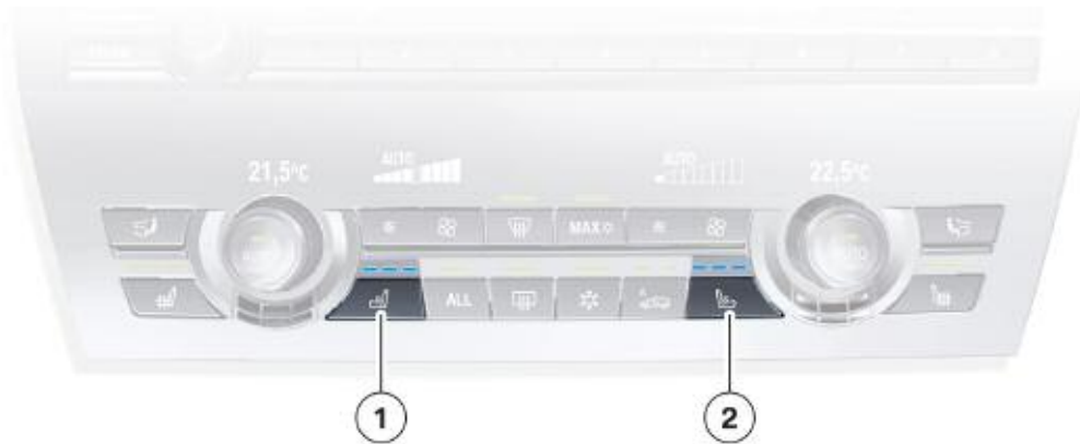
F07 integrated automatic heating and air conditioning system control panel
