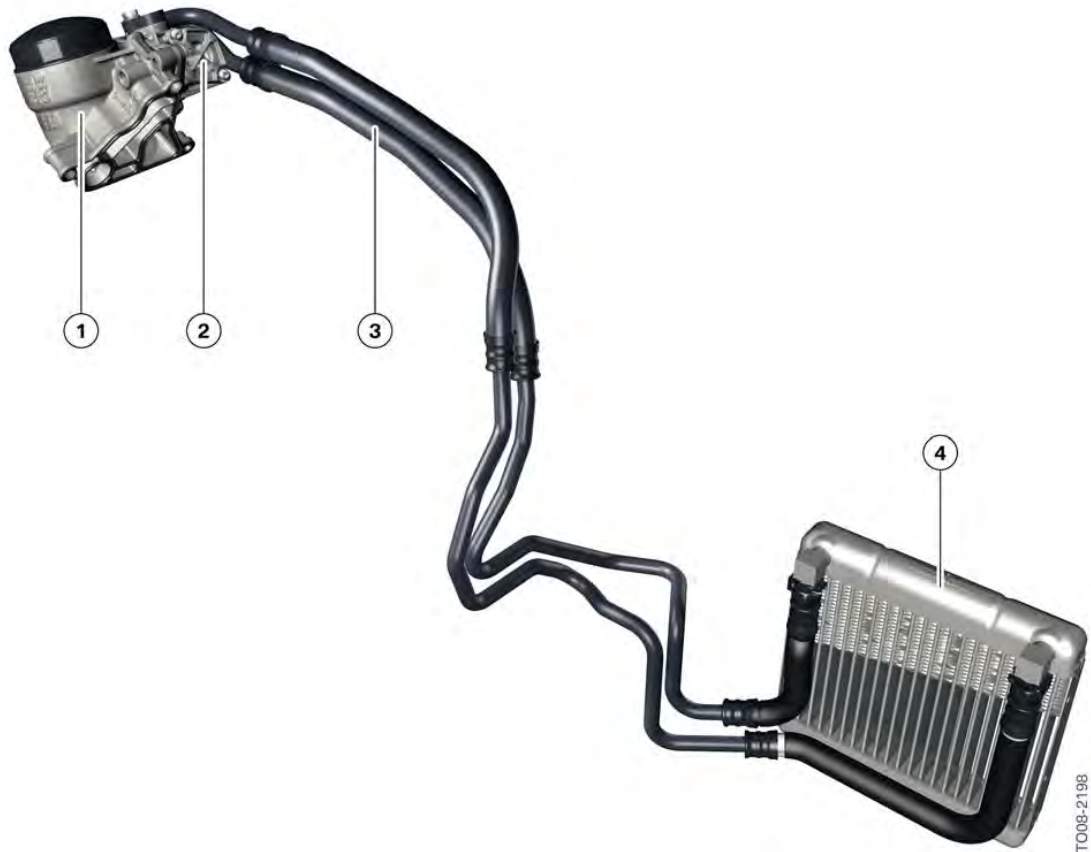
N55 engine, engine oil cooling, hot climate
