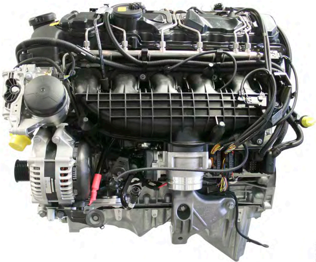
N55 engine, wiring harness routing
