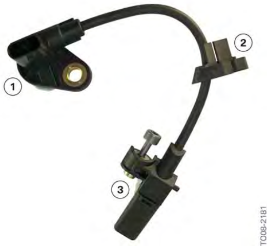
N55 engine, crankshaft sensor with multipole sensor wheel
