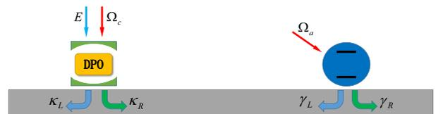
FIG. 1: (Color on line) Schematic diagram of the system. A two-level atom and a single-mode cavity containing a nonlinear medium are dissipatively coupled to a photonic waveguide and are driven by laser fields of Rabi frequencies  $\Omega_c$  and  $\Omega_a$ . The nonlinear medium is pumped with the coupling strength  $E$ .
